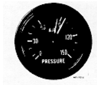
Fig. 3 Air Pressure Gauge
