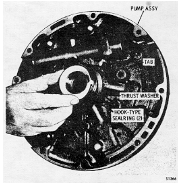
Fig. 7-25. Installing hook-type sealrings onto oil pump assembly
