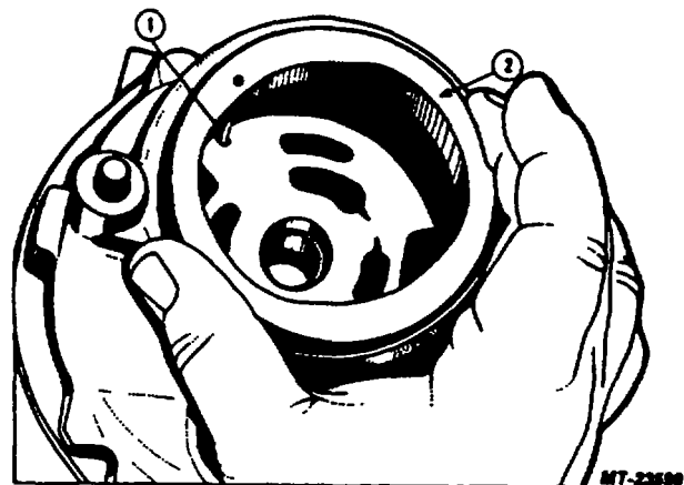
Fig. 31 Installing Cam Ring
