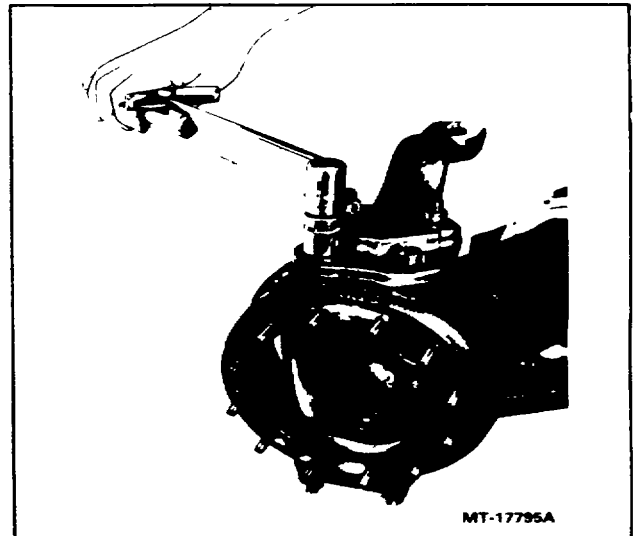
Fig. 20. Checking Bearing Adjustment
