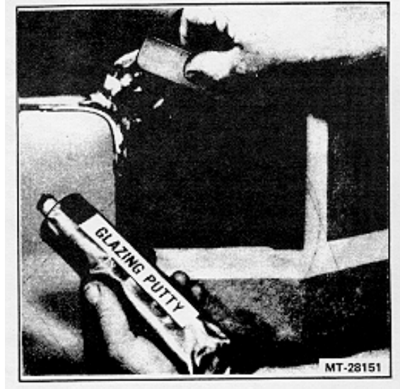
Figure 56 - Applying Glazing Putty
